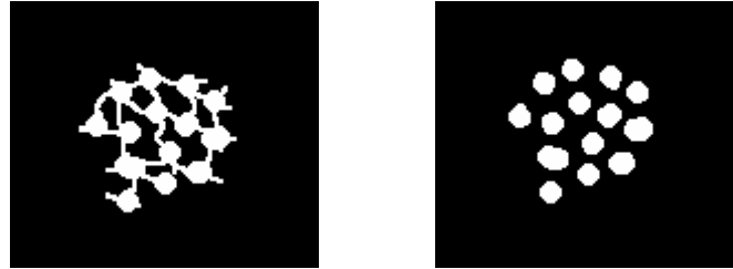
Use of 5 x 5 Octagonal Opening filter to eliminate connections between bright objects
