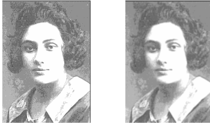
Use of Low-Pass filter to eliminate contouring in a 32 level (5 BPP) Gray Scale image
